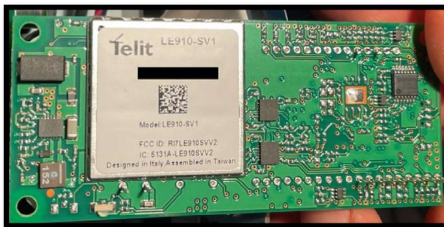
Figure 2 4G Wireless Modem Found Installed On Motherboard of ES&S DS200 Machine
